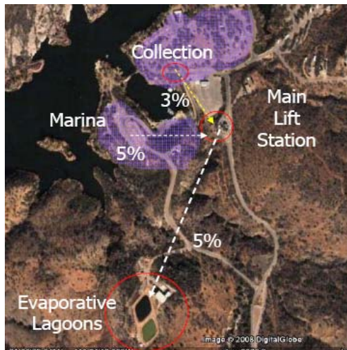
Figure 1: Wastewater System Schematic for Patagonia Lake State Park
